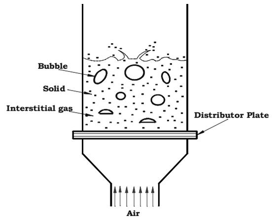
Fig. 3. Bubbling fluidization
