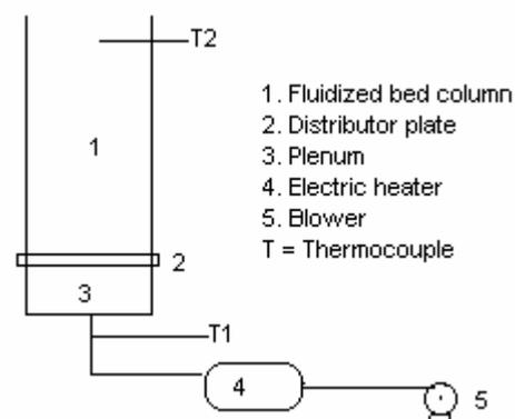
Fig. 1. Schematic of fluidized bed dryer system
