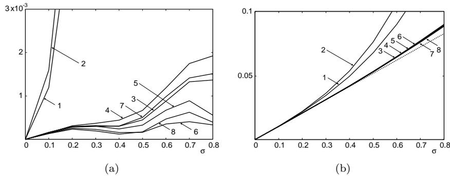
Figure 12: The bias (a) and the RMS error (b) of the computed fundamental matrix for the standard deviation  $\sigma$  (pixels) of the noise added to the data in Fig. 11 over 10000 independent trials. 1) LS, 2) iterative reweight, 3) Taubin, 4) renormalization, 5) HyperLS, 6) hyper-renormalization, 7) ML, 8) hyperaccurate correction of ML. The dotted line in (b) indicates the KCR lower bound.
